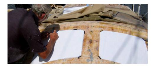
The next part of the job was going to be messy and so Phil took the dodger, now able to stand up on its own safely, down to an empty pontoon, far away from other boats. A 25mm rebate was cut around the external edge of the windows in which to set the "glass".
