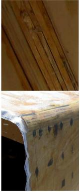
I n order to make rounded corners for the corners of the dodger, Phil cut 10mm strips of plywood, laid them side by side on a length of PVC sewer pipe, held them in place with gaffer tape and then epoxied them up. Allow to dry. The corners were then sanded, put in place and fibreglassed with strips of glass tape and resin.
