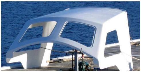
A length of retired jib sheet was used to form a drip lip along the roof edge overhang. This will also serve as a handgrip along the back edge of the dodger. It was continued down the sides to help channel water away from the cockpit. It was screwed on and then given several coats of resin and mat. Allow to dry.
