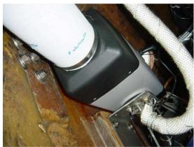
The natural position for the heating unit was the aft lazarette. Not much space left in there after the steering quadrant, hot water system, and port and starboard drogue rodes. Still Mike worked his magic once again and the unit was installed with the ex-
