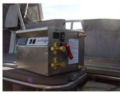
A separate 12v fridge system purchased from Ozefridge in SA was installed in addition to the engine operated system we currently have. The compressor sits in the new machine space starboard aft and a new eutectic plate was fitted in the freezer compartment.
