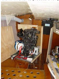
The diesel, named DAPO – short for <u>D</u>iesel <u>A</u>lternator <u>PO</u>wer, is a 2 cylinder Kubota engine with a 210amp Balmar alternator, installed in a sound proof enclosure, which my Captain has made into a work of art. Each panel of the enclosure is interlocking and can be removed for ease of access for the diesel maintenance.
