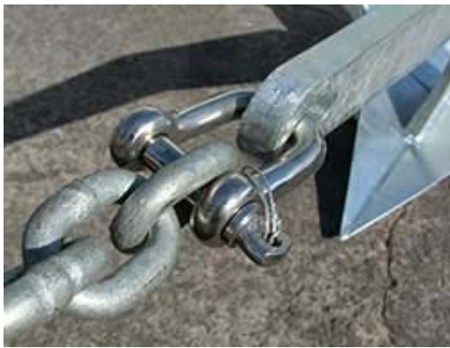
Single shackle between the chain and anchor. Important - always seize the pin
