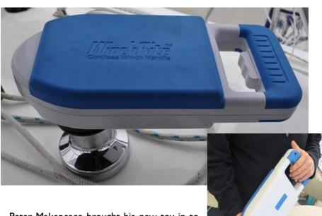
Peter Makepeace brought his new toy in to impress the Editor with – and had me searching the internet for a distributor. This rechargeable device turns all the winches aboard into electric winches. At a cost of \$699 it's not cheap but compare that to an electric winch at about \$1500 – and that's just for one! Local distributor is Ian McConachie at Oyster Cove Chandlery.
