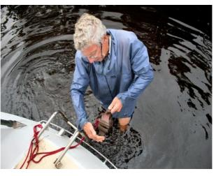
Fitting the vice to the rudder, ready to winch it free
