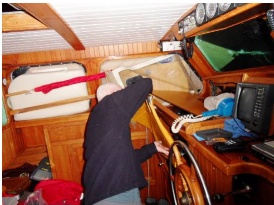
Securing broken pilot house windows
