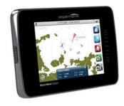
the unit's touch screen. The unit has a built-in GPS antenna, but this did not work where I had my unit mounted – under the steel roof of my dodger. External 'no-name' antennas are available through eBay for only \$5 – rather cheap I thought.
