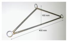
The main bars are 10 mm stainless steel rod and the loops are of 5 mm stainless steel. A couple of possible uses I have come up with are: a coat-hanger for oversized wet-suits; and a spreader bar for lifting the engine out, or for towing a scallop dredge.
