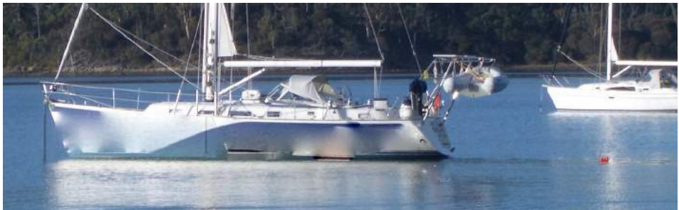
This boat (not Xantia) is close to drifting over its own anchor buoy, potentially fouling its rudder or prop.
