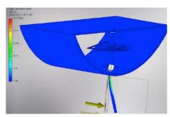
Figure 7. Potential bend in rudder post
