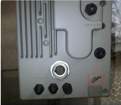
Figure 4: " See ground connection on the rear of Westwind's radar display unit. Ground studs found on electronics are often dismissed, even by professional installers, as unnecessary. Bonding of this equipment is usually mandated by manufacturers.
