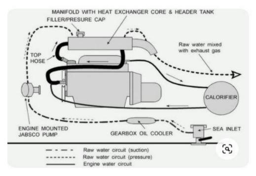
Schematic of a Wet Exhaust system
